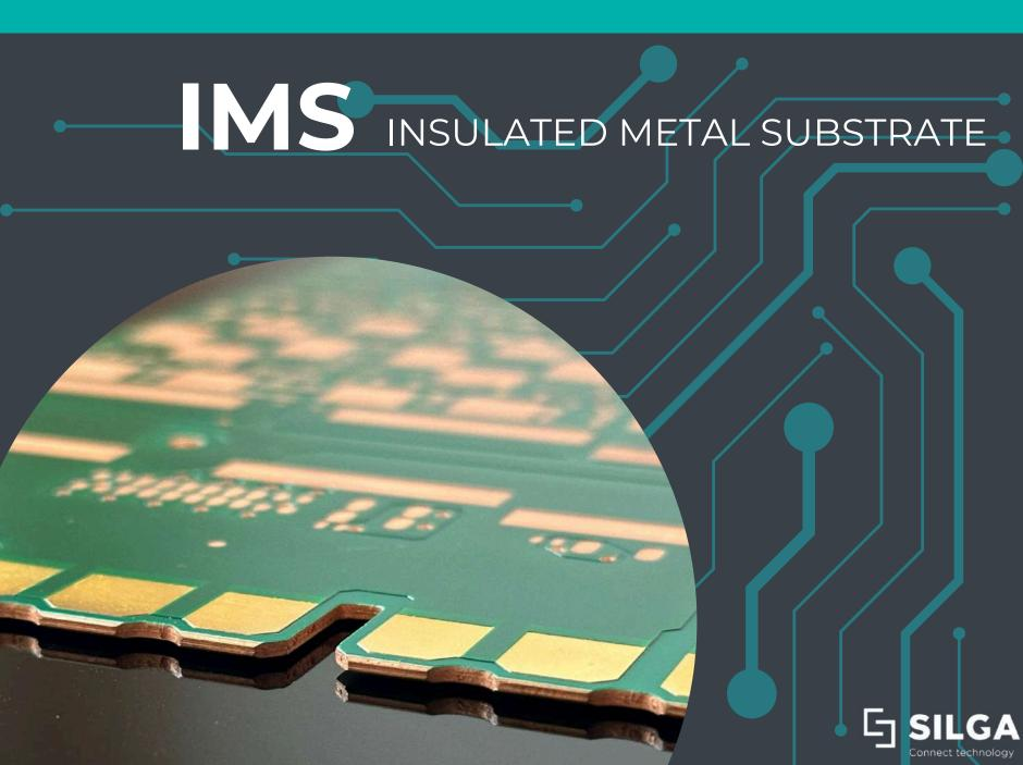
An IMS PCB presents the circuit layer bonded to an electrically insulated metal base to be used for power applications
